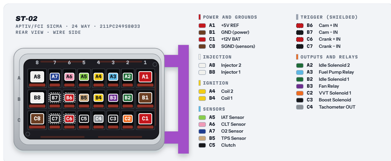
Figure 2.2 ST-02 connector (24-way Aptiv/FCI Sicma) seen from the back: purple lock on the right, row A on top and column 1 on the lock side. Columns 1 and 8 take larger terminals.
