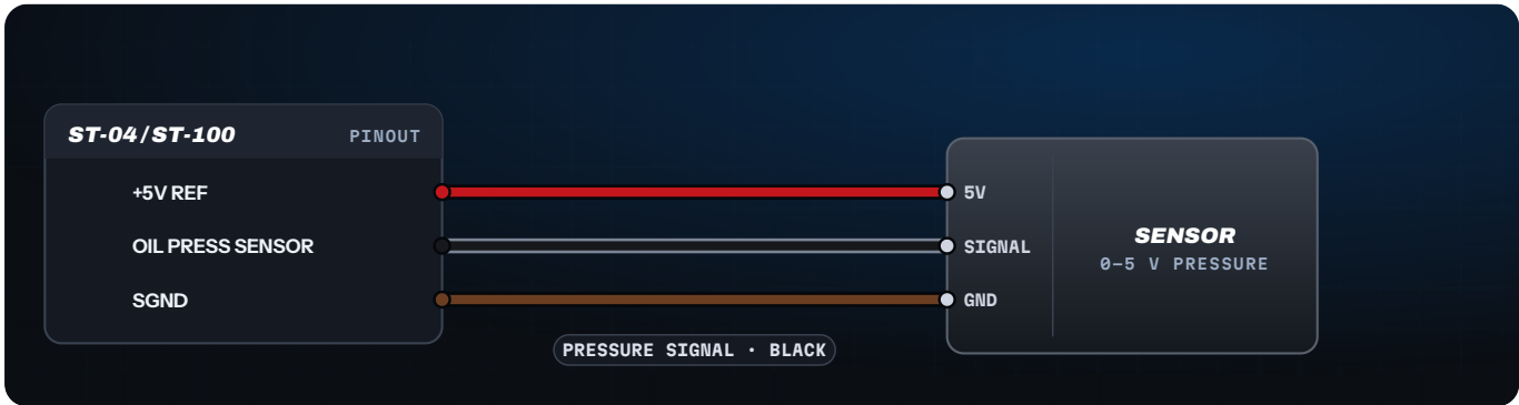
Figure 4.8 Oil pressure sensor on the ST-04 and ST-100 (3-wire, 0-5 V transducer). The fuel pressure sensor connects the same way, with its signal on FUEL PRESS SENSOR. They are enabled in Accessories > Fuel/Oil pressure.
