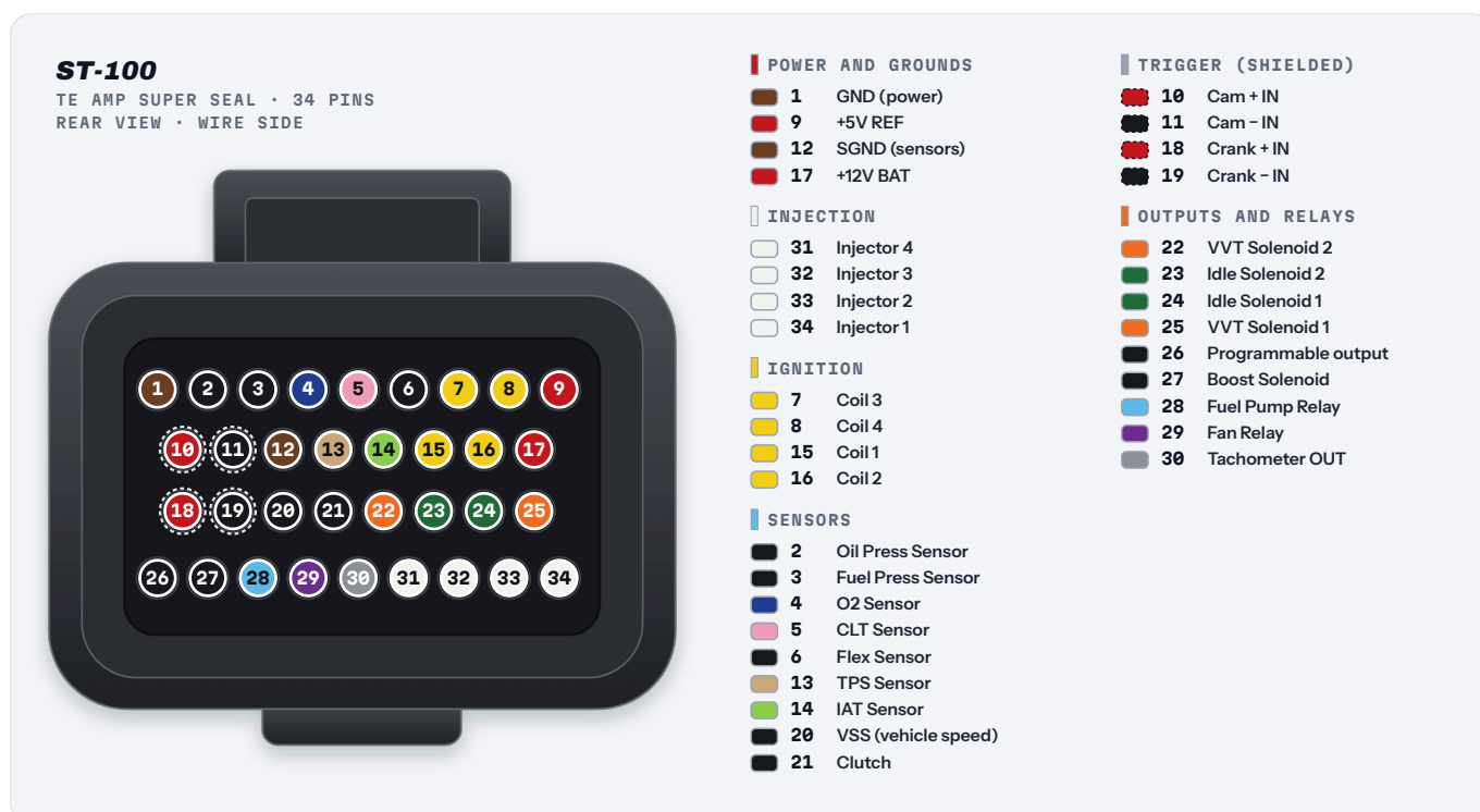
Figure 2.4 ST-100 connector (34-way TE AMP Superseal) seen from the back. The shielded pairs are 10-11 (cam) and 18-19 (crank).
