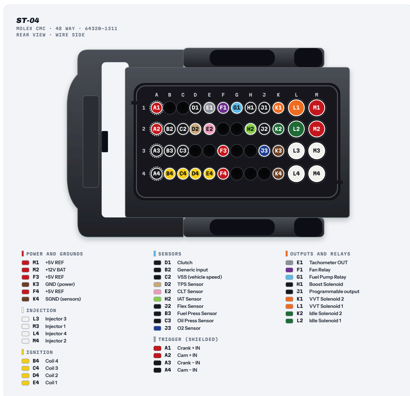
Figure 2.3 ST-04 connector (48-way Molex CMC) seen from the back, with the lever on the left. Columns L and M are the large cavities, for power and injectors.
